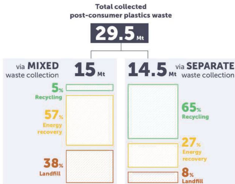
Figure 8: Fate of plastics for mixed and separated waste collection in Europe (Plastics Europe 2022)
