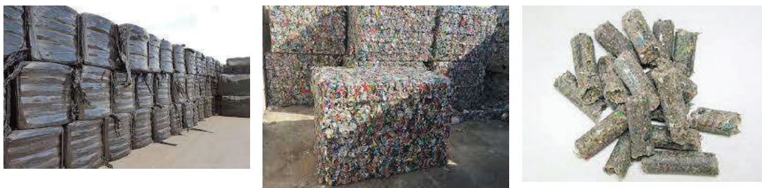
Figures 14: RDF forms (wrapped bales, metal strapped bales and pellets)
