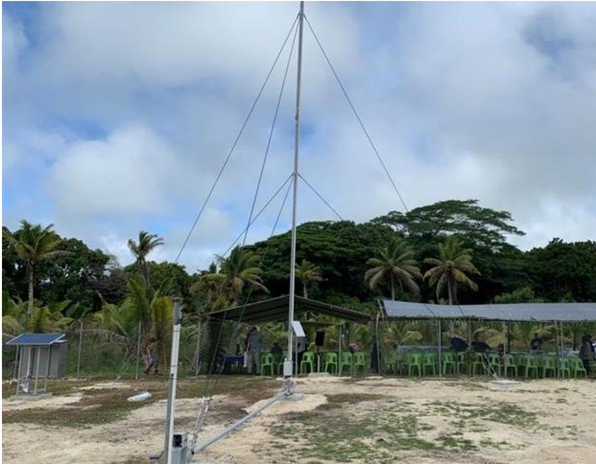
Automated Weather Station in Niue, Pacific Programme
