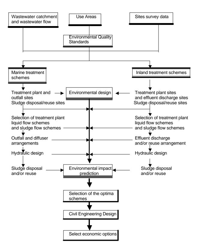
Figure 4. Wastewater sanitation schemes - design flowchart
