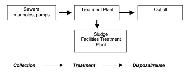
Figure 1. Wastewater sanitation system components
