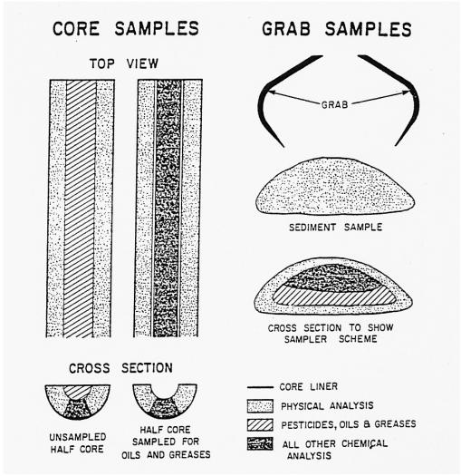
Figure 5: Collection of sediment according to analysis required.
