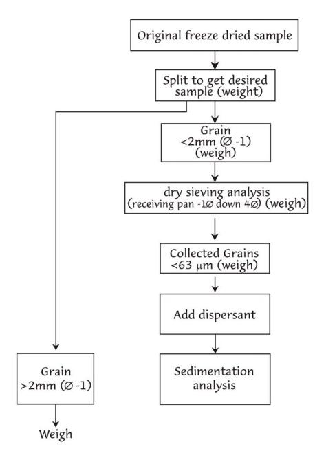
Figure 6: Sequence of steps for the grain size separation of a sediment sample (Please note that 2mm grain size stands also for one mm).
