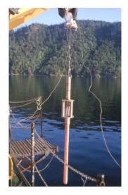
Gravity core sampler (picture: S. de Mora)
