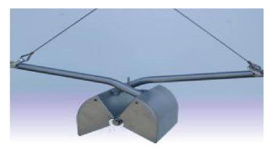
Figure 1: Van Veen grab operated manually (picture from Hydro-Bios, Germany).
