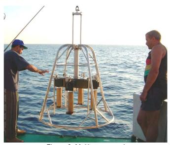
Figure 3: Multi-core sampler.
