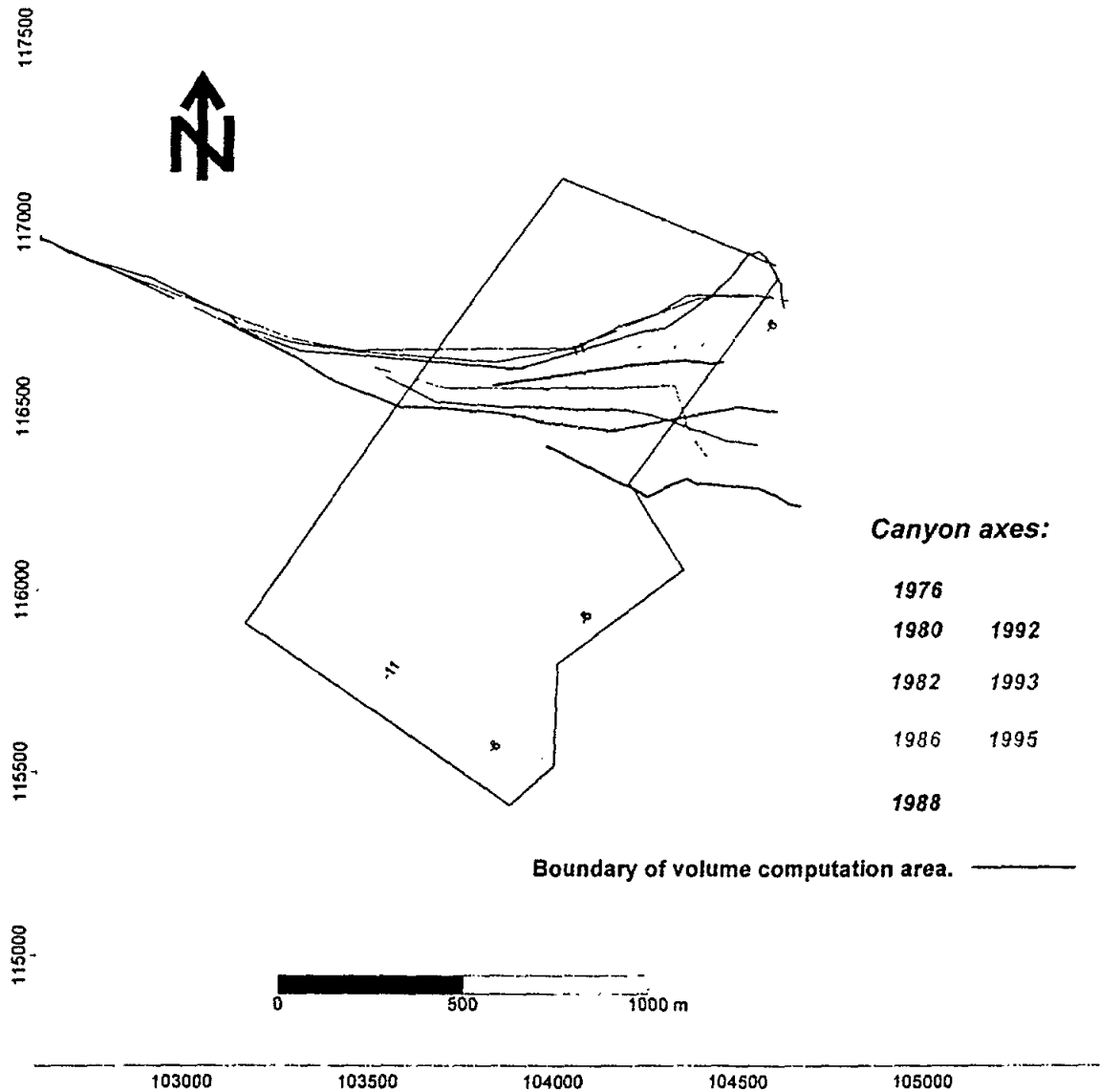
Figure 24. Positions of canyon axes, offshore Rutenberg cooling basin, between 1976 and 1995, and area used for volume computations.
