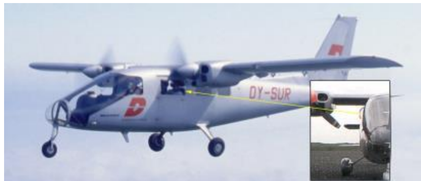
Fig. 5. Partenavia P-68 Observer aircraft with bubble window
