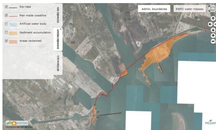
Fig 3. Inventory of manmade coastline and areas reclaimed (French Mediterranean coast). Source: MEDAM 8
