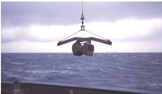
Large grab sampler (picture: S. de Mora)
