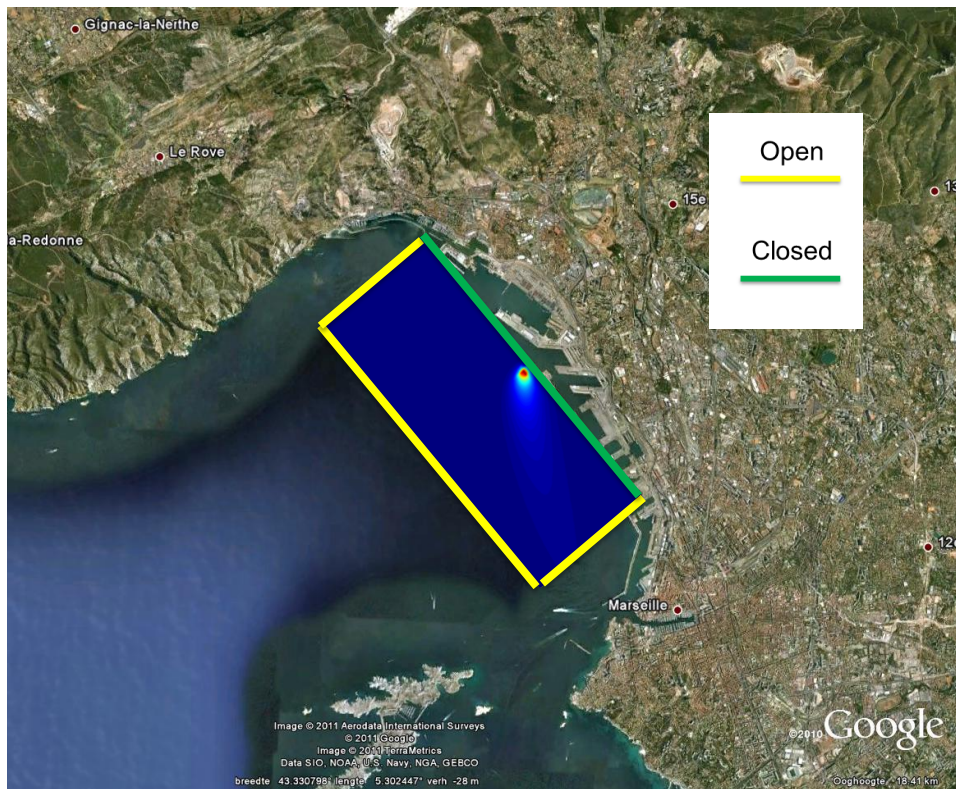
Figure 3.1 Top view of a simplified rectangular representation of an “open” environment; example of an “open” environment for the Gulf of Lions (Deltares, 2012)
