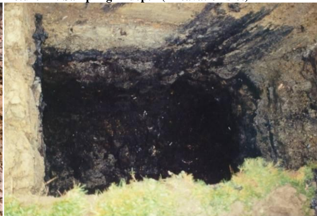
Picture 22: Sampling in depth (Excavation slot)
