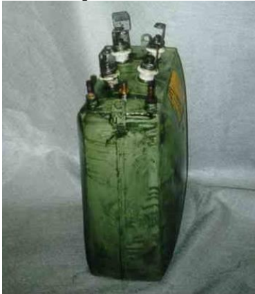
Picture 42: Inflated capacitor
