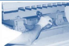
Sample the oil (30-50ml for PCB screening, 1 if also oil quality is tested)
