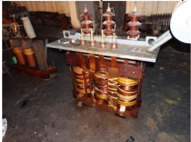
Picture 41: Active transformer part in Albanian workshop
