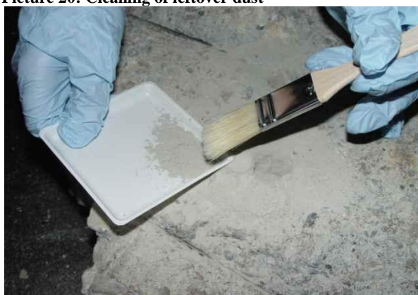
Picture 20: Cleaning of leftover dust
