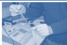
Screen the oil sample by Clor-N-Oil or L2000 DX Analyzer (on site or off site)
