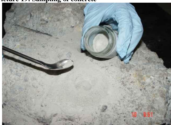
Picture 19: Sampling of concrete
