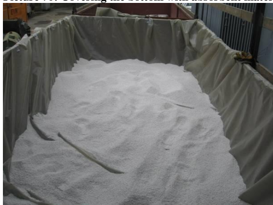
Picture 70: Covering the bottom with absorbent material
