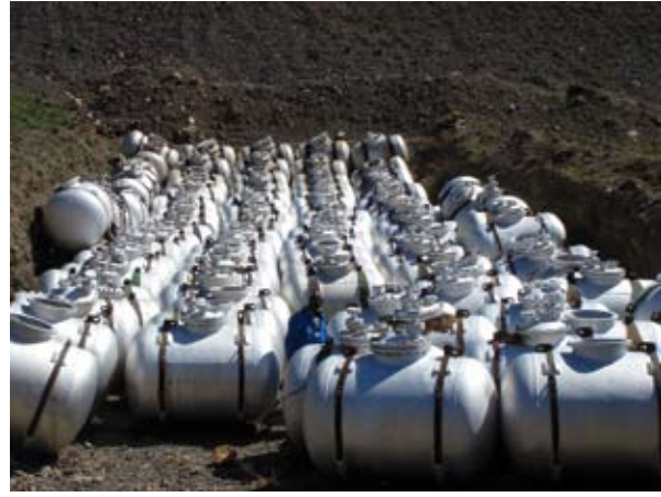
SCUD missile fuel containers stored below ground level in a shallow trench.
