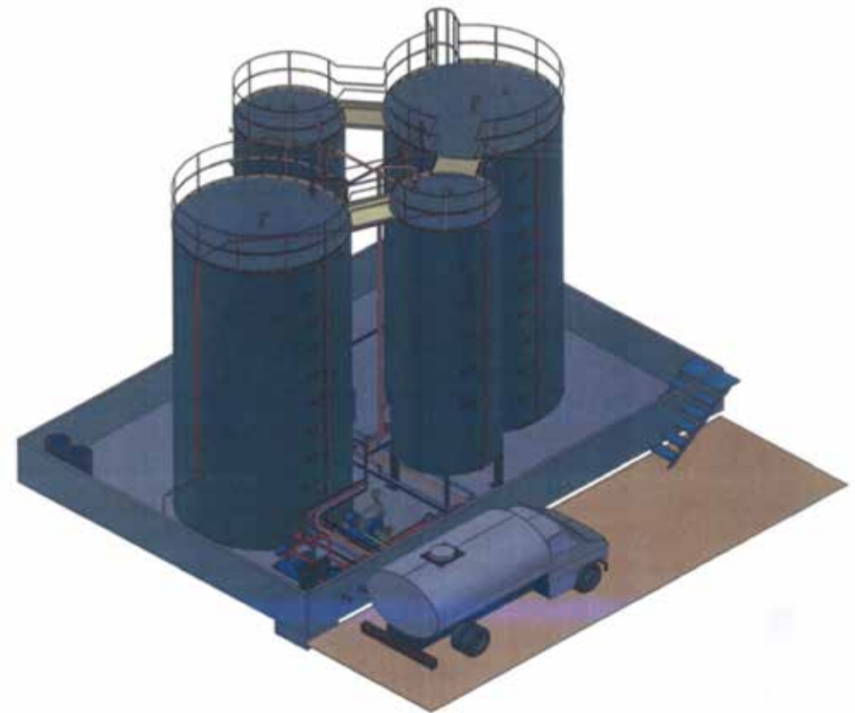
Example of transfer centre with a storage capacity for used oil of 260 m 3
