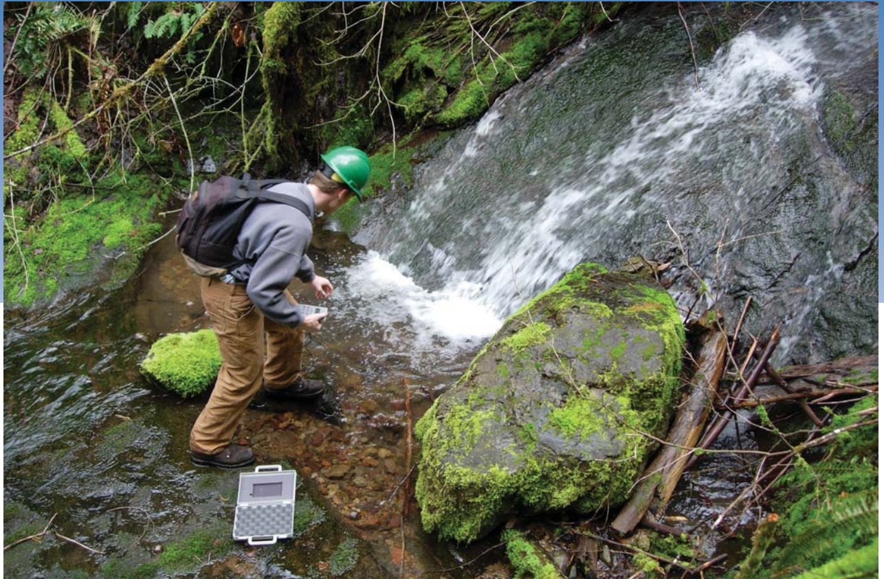
Student measures stream electrical conductivity in the western Cascades during an OSU Field Hydrology class. Photo credit: Jeff McDonnell.
