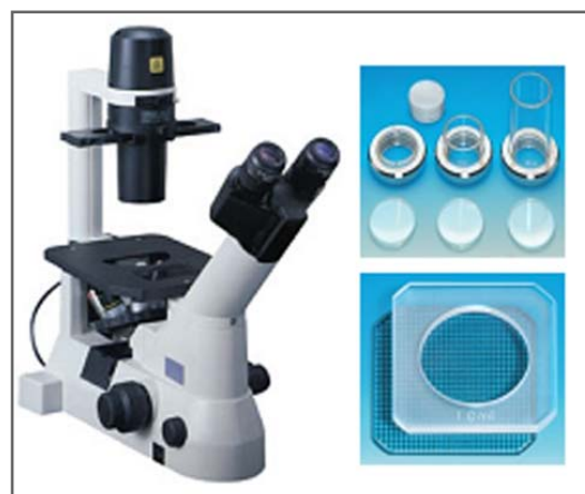
Fig. 7.5 Utermöhl counting technique using a counting chamber and inverted microscope. (photo: Department of Applied Ecology)
