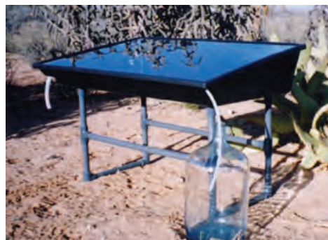
Figure 11 Model of solar stills (SolAqua, 2009)
