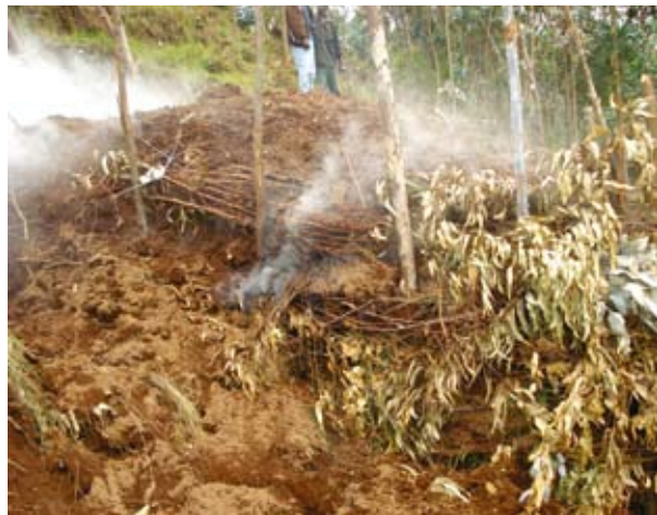
A traditional kiln for burning charcoal – they are quite inefficient using a lot of wood contributing to deforestation
