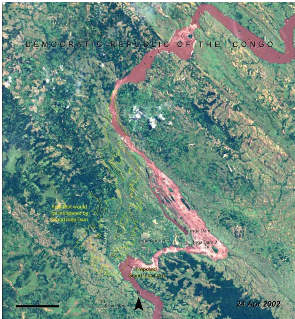
Figure 2.2.6: The reservoir of the proposed Grand Inga Dam would submerge roughly 55 km 2 of land if the project were to go forward as originally designed
