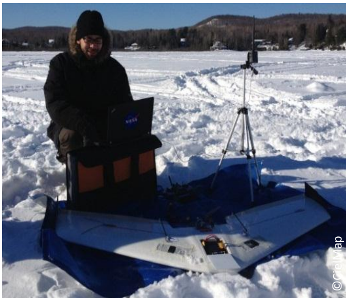
Figure 2. A prototype of a CielMap drone (left image) and a sample high resolution image (right image) taken with the 12 MP camera on board.
