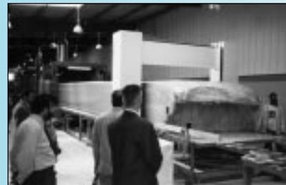
The Kolaghassi Foam and Mattress Factory Co. (Amman, Jordan) demonstrating the manufacture of non-CFC flexible polyurethane foams for mattresses to members of the West Asia Network of ODS Officers. This completed investment project, replacing CFC-11 with methylene chloride (JOR/FOA/07/INV/08), was implemented by the World Bank and resulted in the elimination of 20 tonnes of CFC consumption.
