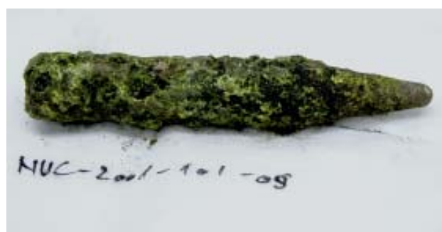
Corroded penetrator collected at Pljackovica
