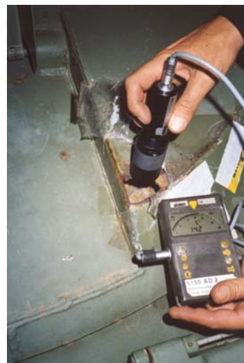
Measuring beta and gamma radiation from penetrator hole in APC at Vranje Garrison
