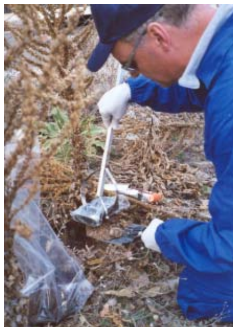
Beta and gamma measurements on soil sample from penetrator hole at Pljackovica
