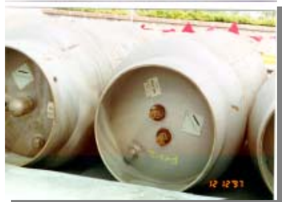
Photo 4: View to the access valves of the small HFC-134a containing cylinder.
