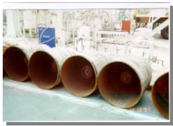
Photo 2: View of the small HFC-134a cylinders after removal of the CFC-12 refrigerant and cutting open the main containers.
