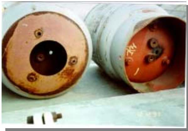
Photo 1: The access points to the main CFC-12 container only become visible after cutting open the double layered container.
