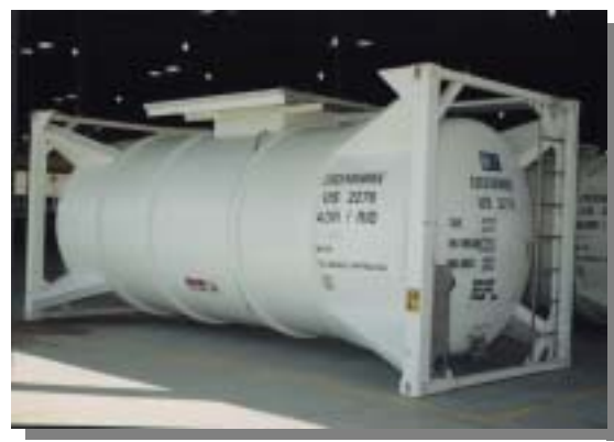
Photo 24: ISO tanks allow for multimodal transport of large quantities of refrigerants.
