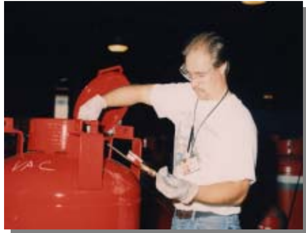
Photo 29: Conducting a temperature/pressure test
