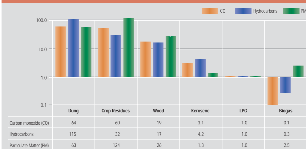
Figure 4: The energy ladder: relative pollutant emissions per meal with LPG* set to 1.0
