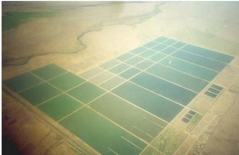
Figure 5: Stabilization ponds as appropriate technology in developing countries (Dandora Treatment Works, Nairobi, Kenya)
