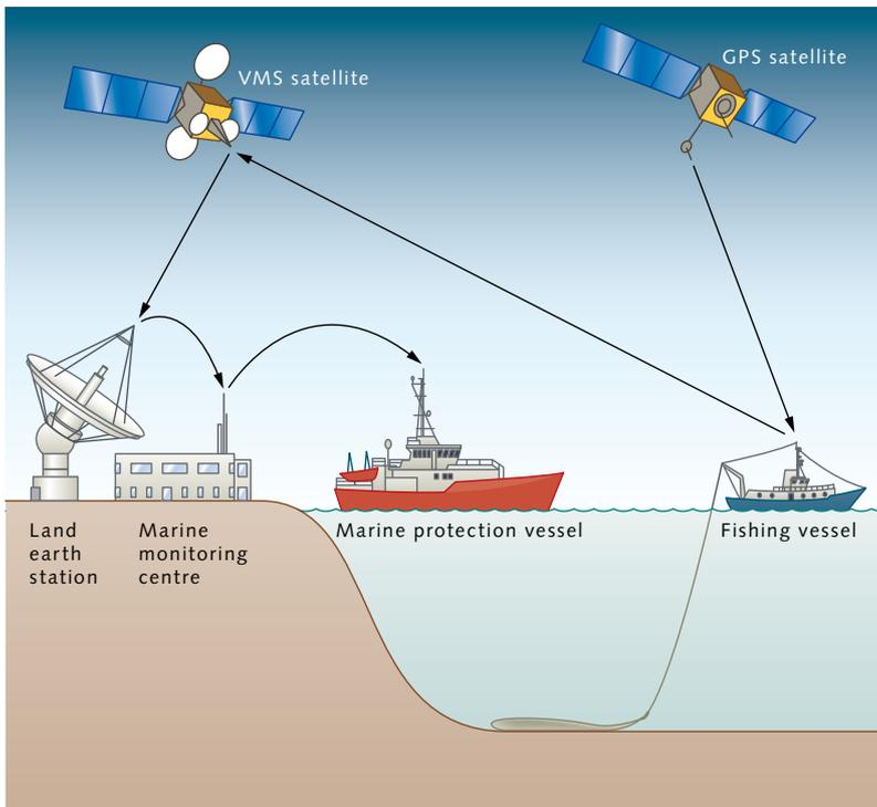
**3.28 > Nowadays, fishing vessels must be equipped with electronic devices, or “blue boxes”, which form part of the satellite-based vessel monitoring system (VMS). The blue box regularly sends data about the location of the vessel to the fisheries monitoring centre (FMC). Vessels are also equipped with GPS transmitters which track the ship’s speed and position.**
