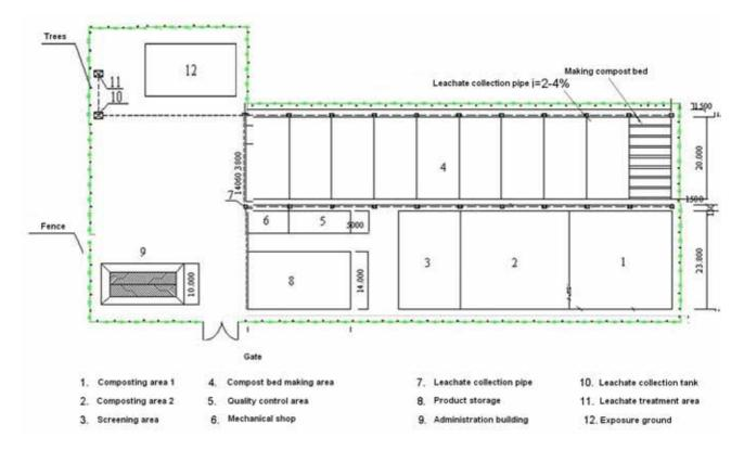
Figure 8 Layout of Composting Plant
