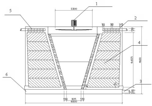
Figure 4 Details of cooling tower
