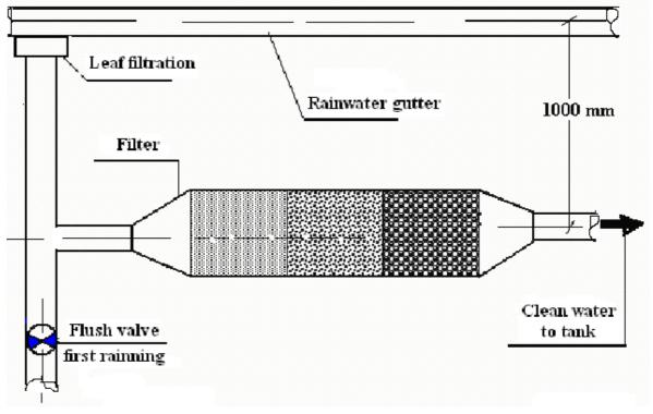
Figure1 Rainwater harvesting system for Song Cong Sugar Company
