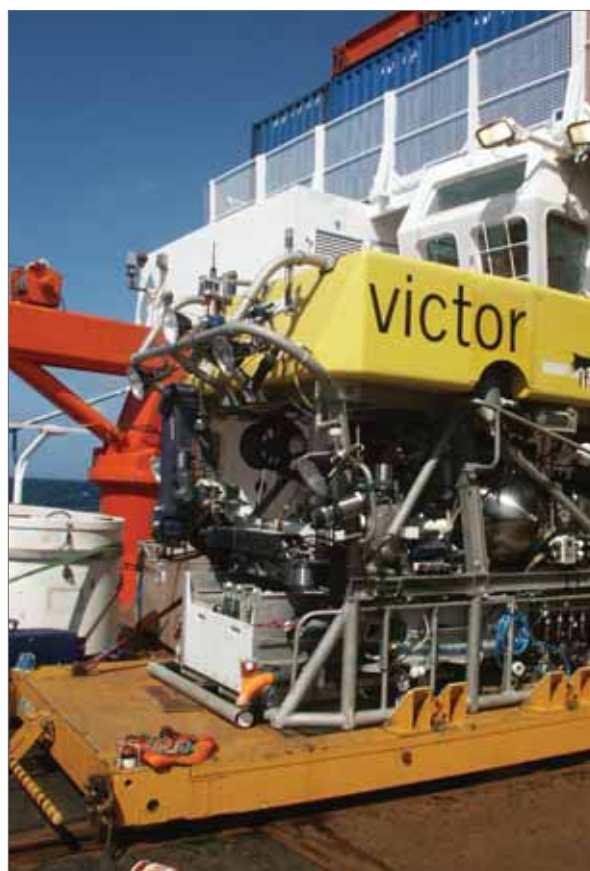
Figure 2.5: The Victor remotely operated vehicle from the French marine research institution Ifremer. J.M. Roberts.
