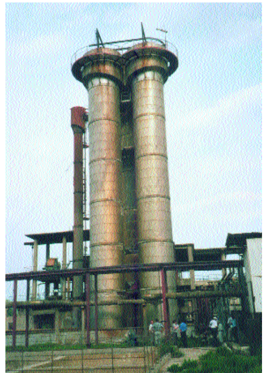
Steel columns containing arsenate and arsenite solution, Fier
