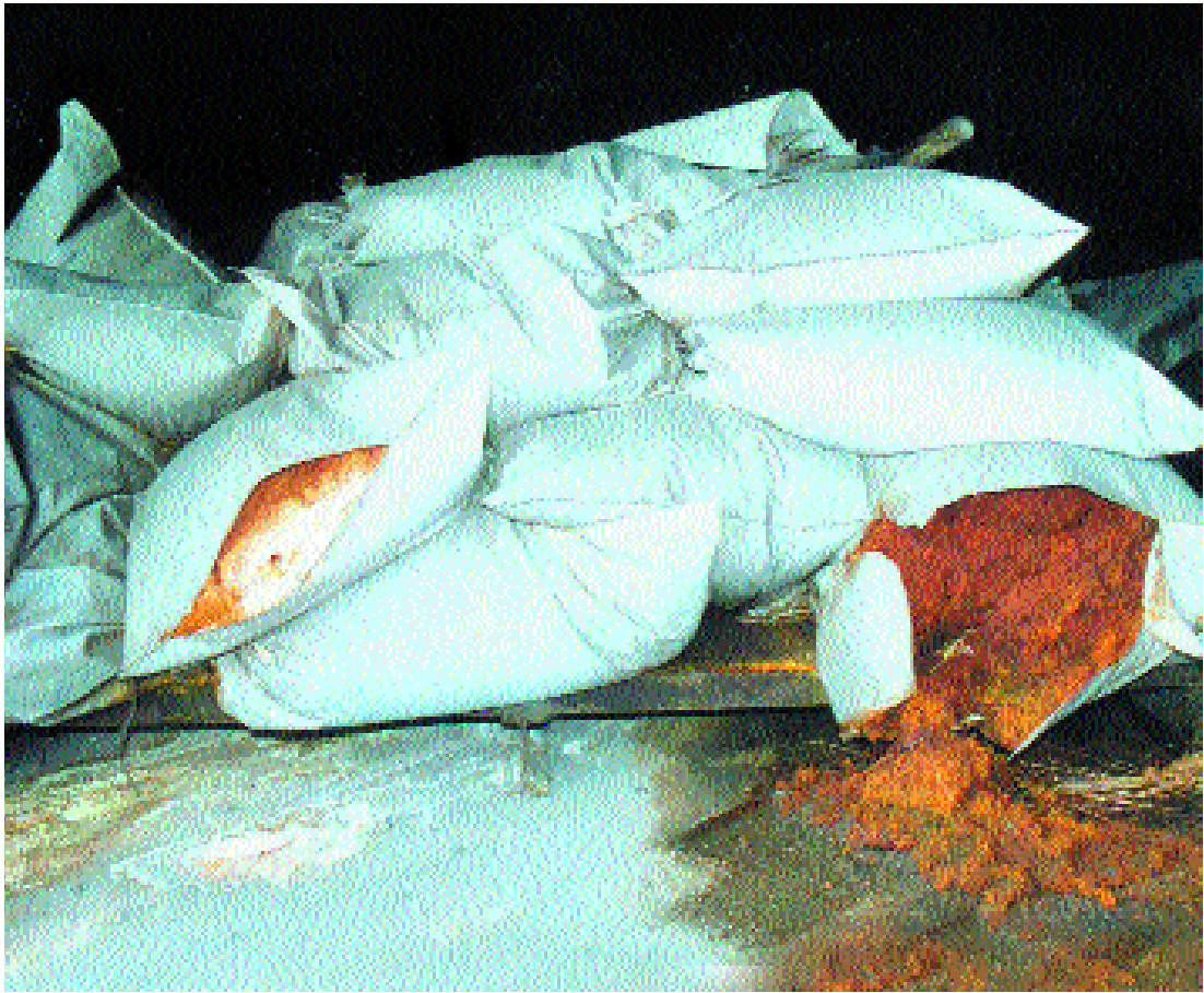
Improperly stored hexavalent chromium compounds at HEK Jugochrom
