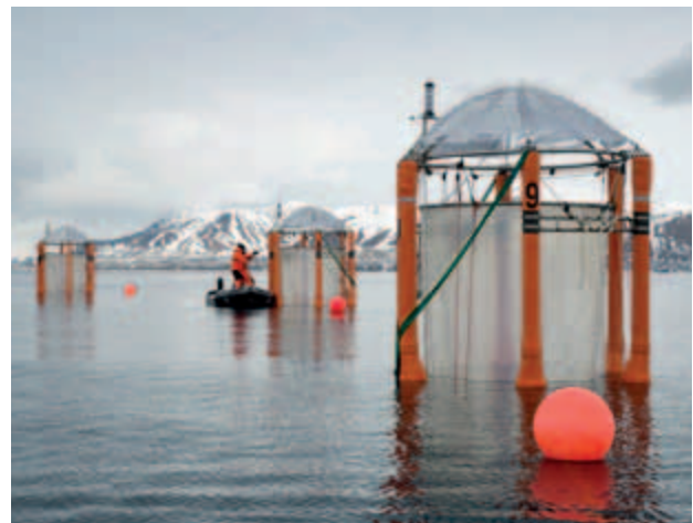
Figure 3.5. Two experimental approaches to investigate the impact of ocean acidification on marine species: laboratory-based perturbation experiments (left, Maj Arnborg) and large-scale field-based mesocosms (right, Maike Nicolai).
