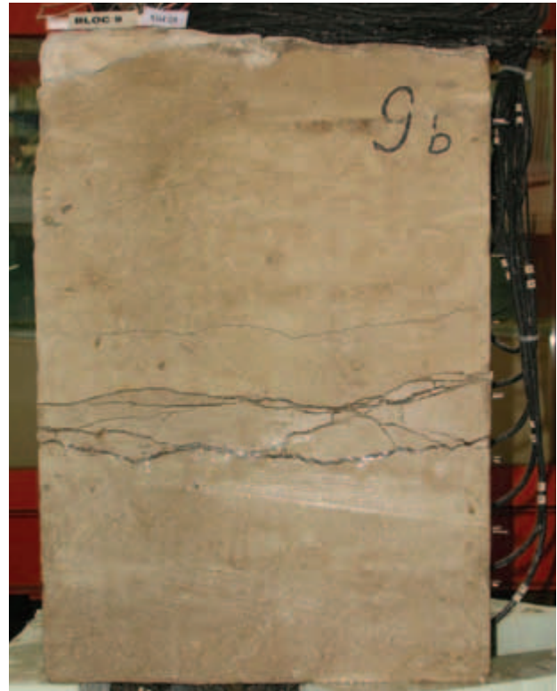
Figure 5.23. Fractures formed by ice segregation in Totternhoe Stone (a type of English chalk) following twenty-four cycles of bidirectional freezing of an active layer above permafrost. The fractures are filled with segregated ice and occur primarily in near-surface permafrost and at the base of the active layer. Some narrow cracks are also visible in the upper part of the active layer, caused by downward freezing from the rock surface. The block is 450 mm high and 300 mm wide. Photo Julian Murton, University of Sussex, UK.
