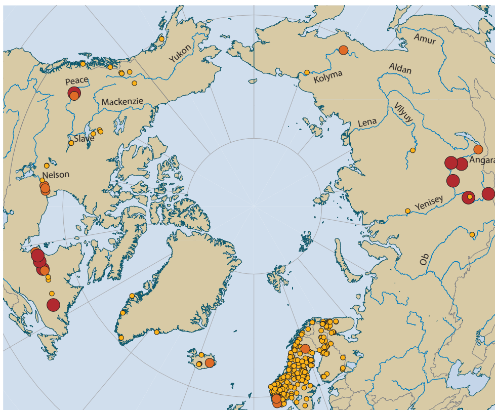
Figure 6.23. Location and size of major hydroelectric facilities located in ice-dominated river regimes of the circumpolar North. All such stations will require major modifications to current operational regimes and possibly infrastructure modifications based on projected changes to freshwater ice regimes (due to data availability, the figure may not show all existing plants). Source: Knut Alfredsen, Norwegian University of Science and Technology, Trondheim.
