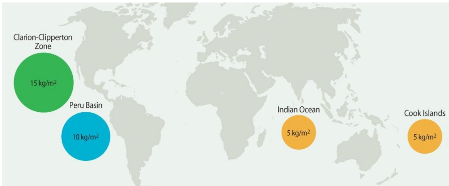
Figure 4. Average abundance of polymetallic (manganese) nodules in four major locations (GRID-Arendal adapted from Hein et al., 2013).
