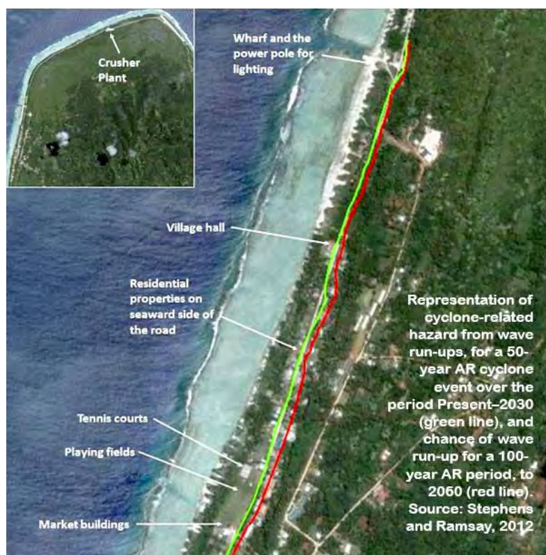
FIGURE 3.4. Coastal areas near Oneroa village (Cook Islands) showing key community facilities at risk from coastal inundation under different scenarios using the Cook Islands Coastal Calculator.
