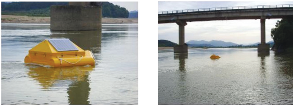
Figure 4: IP-USN installed at the Sangjubo station (downstream from the Jeongdong Bridge)
