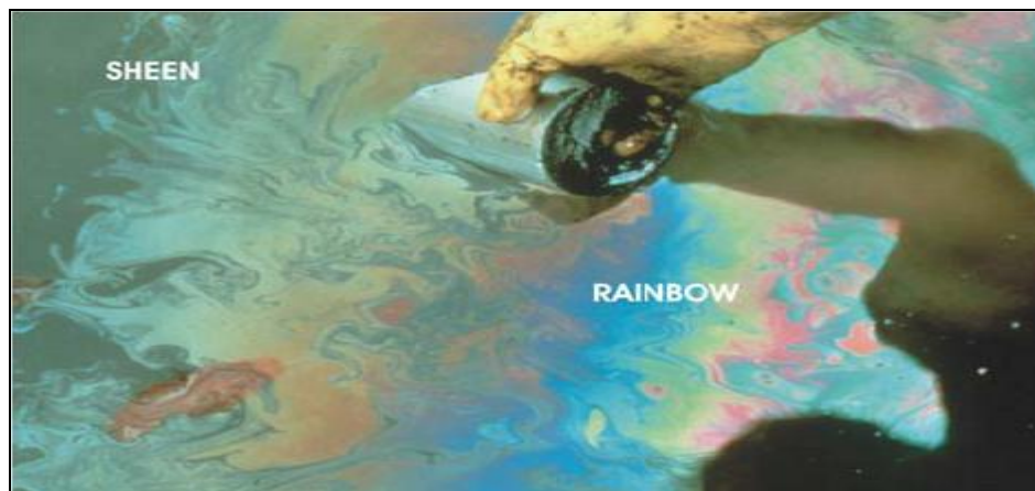
Figure 14: A photograph of sheen and rainbow oil. The thickness of this oil is less than 0.001 mm (1 µm) (Source: "Oil on water sheens" – Ron Goodman Innovative Ventures Ltd)
