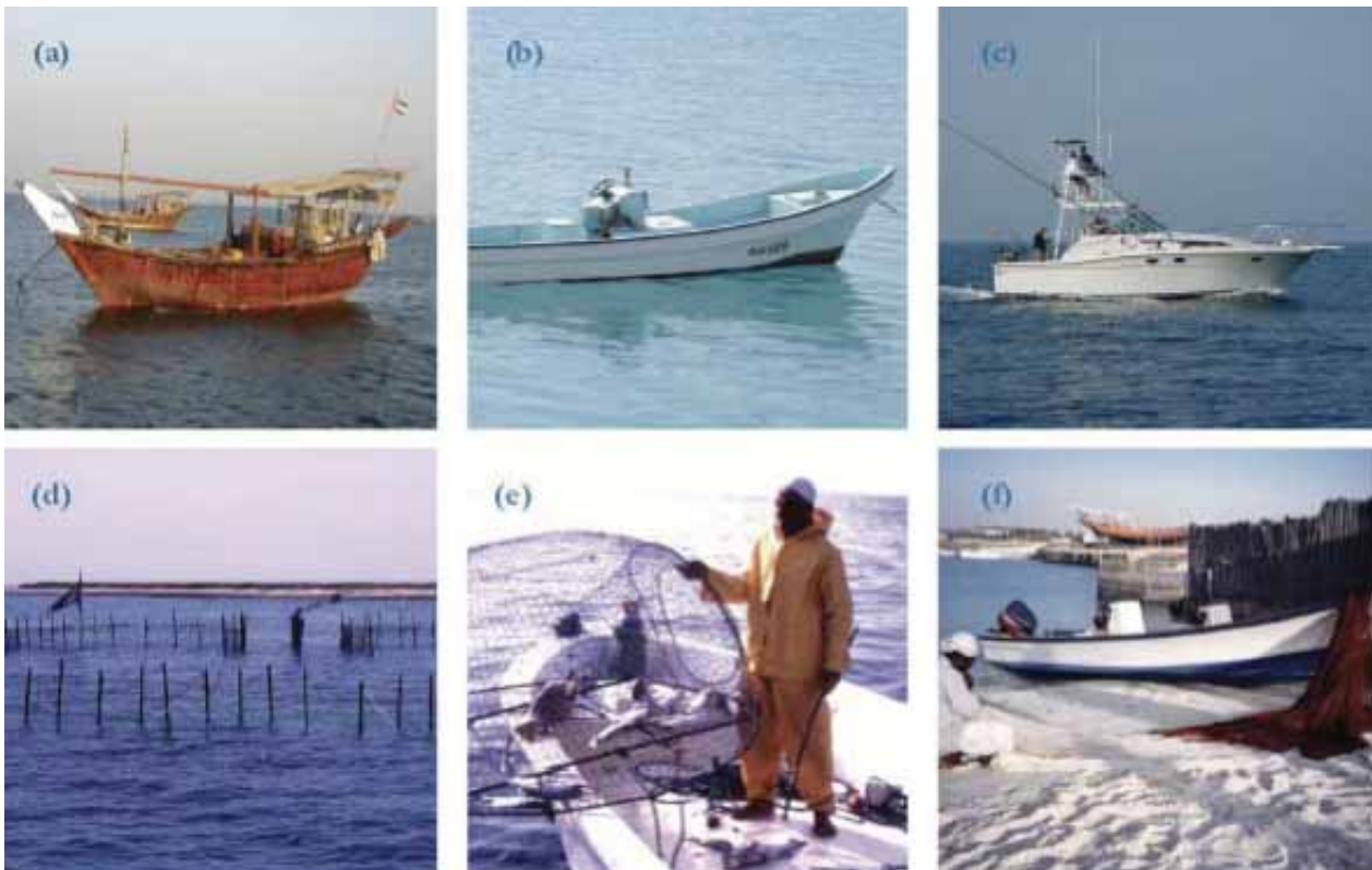
Figure 47: Some of the fishing vessels and gears used in Abu Dhabi (a) traditional dhow or 'lansh' (b) dory or 'tarad' (c) recreational (sport) fishing vessel (d) inter-tidal fence net 'Al Hadhra' (e) wire trap 'gargoor' and (f) encircling gillnet.
