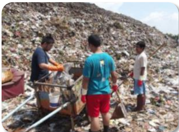
Waste composition is sampled to improve accuracy of GHG emission calculations as part of the MRV system of the v-NAMA project in Indonesia, coordinated by GIZ (see 4.5). Photo: V-NAMA Indonesia
