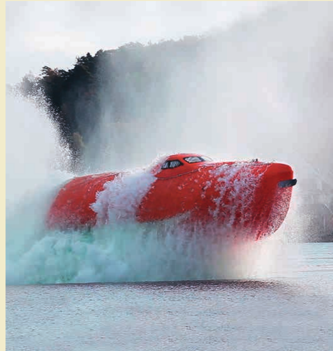
3.6 > Endurance test of a rescue boat: under the SOLAS Convention, lifeboats must undergo certain checks. One of these is the drop test, where a fully-loaded lifeboat is dropped into the water from a height of several metres.
