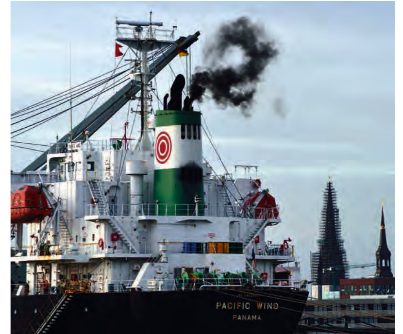
4.8 > Exhaust gases from shipping are a problem in many ports, such as Hamburg (above). Under IMO rules, these exhaust gases will contain lower levels of pollutants in future. Black smoke cannot be avoided altogether, however: it is emitted in short bursts from ships' revving engines during docking.
