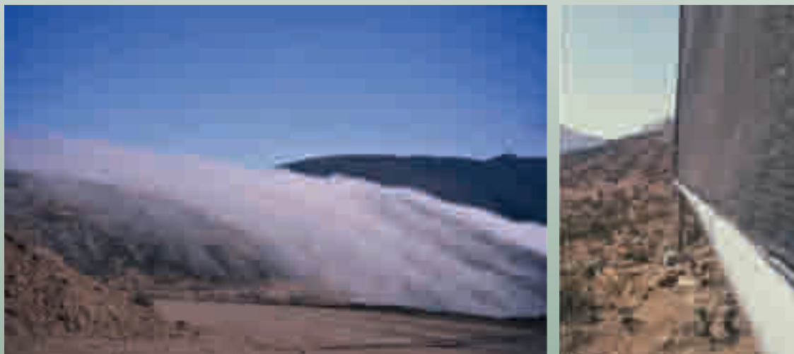
Fog and fog collectors in Chile. Fog ( camanchaca ) is common on the coast of the Atacama Desert, between, 8°S and 32°S, as in some other coastal deserts. The experiment with the fog collectors was to see if they could produce enough water for livestock, afforestation, water supply and wildlife.
