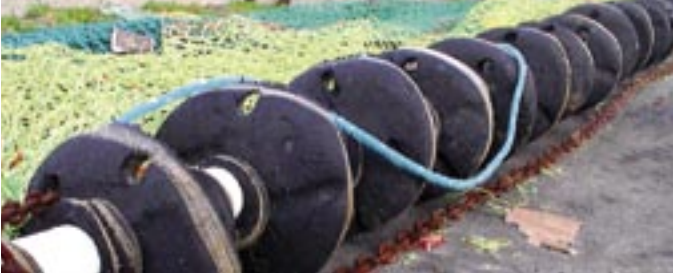
Bottom trawl roller-gear Source: © OCEANA / David Hall
