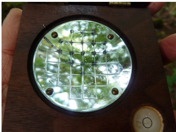
Figure 3: An estimate of canopy cover is taken using a densiometer. The observer is required to score the amount of canopy cover reflected in each of the 24 squares marked on the mirror surface.
