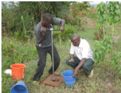
Figure 3. Metal sampling plate with auger placed in center hole (Photo from AfSIS)
