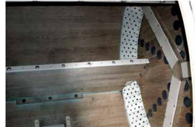
Fig 3: Cangilones off-centre shelves (not looking to the axle) enable hides and float to be lifted to the highest level inside the drum before dropping this mass on top of other hides, creating the «sponge effect».
