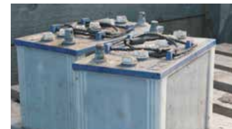
Fig. 46: Examples of bad used lead batteries management
