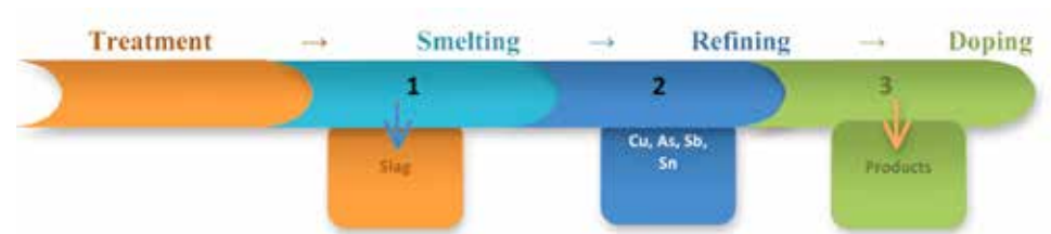
Fig. 18: Typical used lead batteries recovery process 10
