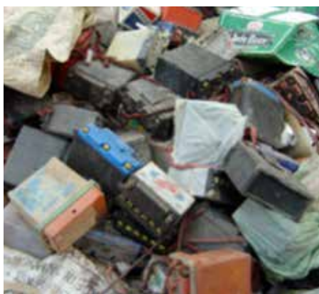
Fig. 10: Bad examples of used lead batteries collection 25
